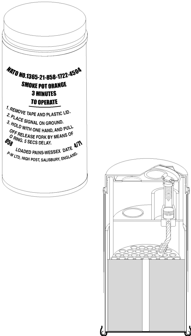
Figure 5-3: Smoke pot, ground type, orange, 3 minutes
